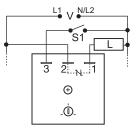
S1 = Optional low current switch V = Voltage L = Load
