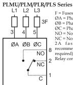
F = Fuses  $\emptyset$ A = Phase A = L1  $\emptyset$ B = Phase B = L2  $\emptyset$ C = Phase C = L3
