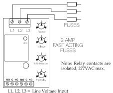
NO = Normally Open Contact NC = Normally Closed Contact C = Common, Transfer Contact
